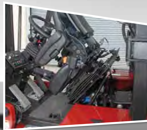
Tilting operator seat gives easy access to drivetrain components.
