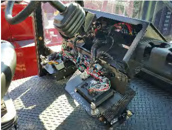
Flip-down Dash with Color/Number Coded Wiring (Standard)
