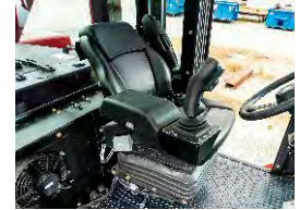
Fully Adjustable Air Ride Seat (Standard)
