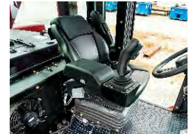
Fully Adjustable Air Ride Seat (Standard)
