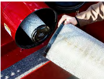
Donaldson Air Cleaner with Safety Element (Standard)
