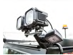
12 LED Work /Step Lights (Standard)
