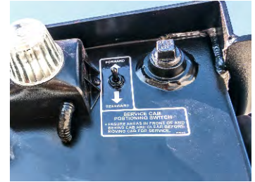
Service Cab Positioning Switch allows the Cab to be Traversed with Machine Powered Down
