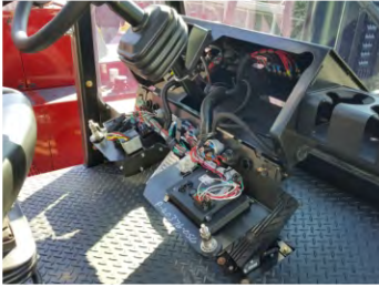
Flip-down Dash with Color/Number Coded Wiring (Standard)
