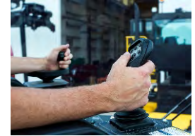
Mini-Wheel Steering & Joystick Control (Standard)
