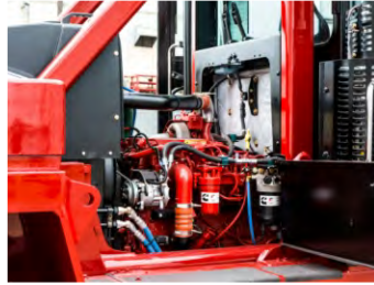
Easy Access to Drive Train & Hydraulics
